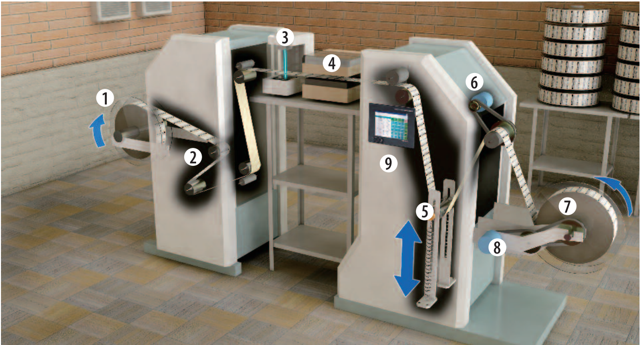
Easily integrate sequence and motion control with an FX PLC: ① Unwinding reel. ② Reel size compensator. ③ Start/Stop sensor. ④ Printing device. ⑤ Dancing roller. ⑥ Drive train. ⑦ Winding reel. ⑧ Winding motor. ⑨ Control panel
