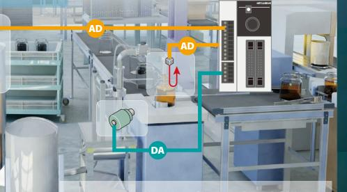
Typical application for level and filling control based on analog measurement.
