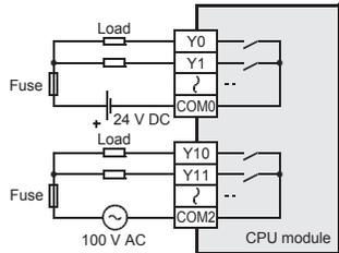
3.6 Transistor output specifications and external wiring
