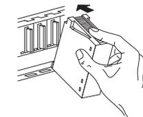
② Push the module in the direction of arrow to load it into the base unit.
