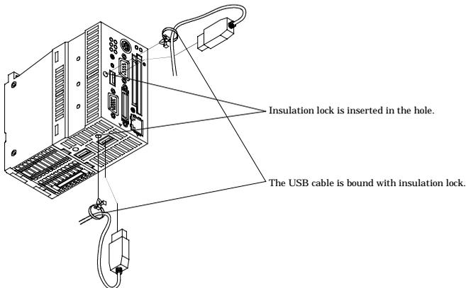
**Figure 5.5. Insulation lock attachment hole**
