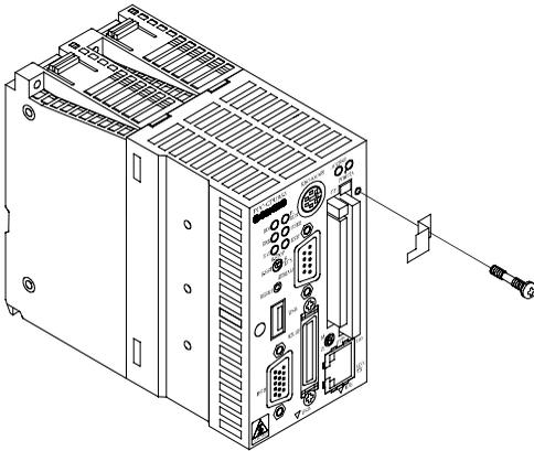
**Figure 5.4. Attaching a Card Stopper**
