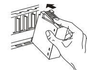
③ Secure the module with an additional screw (M3 x 12) to the base unit if large vibration is expected. This screw is not supplied with the module.
