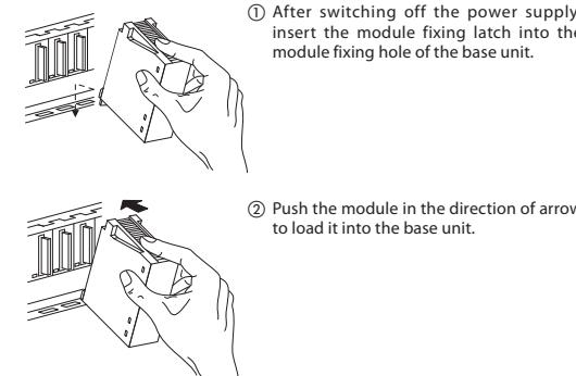
① After switching off the power supply, insert the module fixing latch into the module fixing hole of the base unit.
