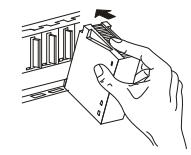
② Push the module in the direction of the arrow to load it into the base unit.
