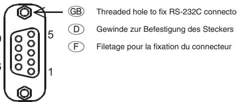
**(GB)** Please note that a inch screw thread (#4-40UNC) is used to fix the connector to the QJ71PB92D.
