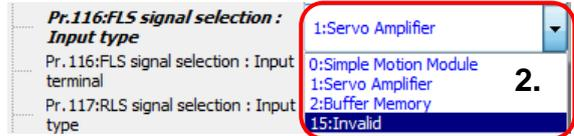
Set common/basic/detailed/home position return/expansion parameters where necessary. (Refer to Appendix 2 for setting examples.)
