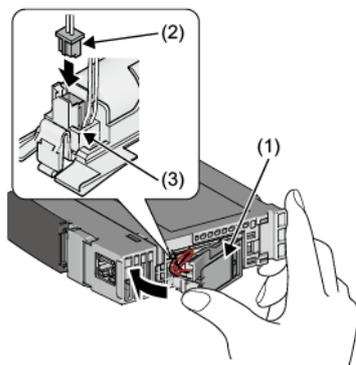
1. Open the battery cover located on the bottom of the CPU module.
