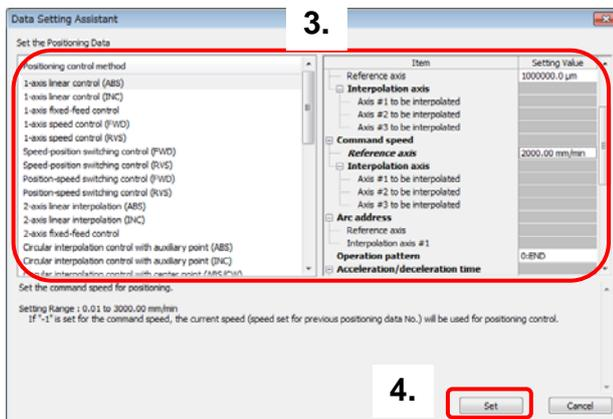
Positioning control method: 1-axis linear control (ABS)
