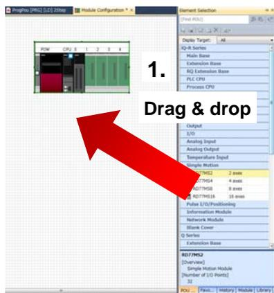
1. Select the main base unit, CPU, I/O, and Simple Motion module to be used from the POU list, and drag & drop them to the configuration screen.
