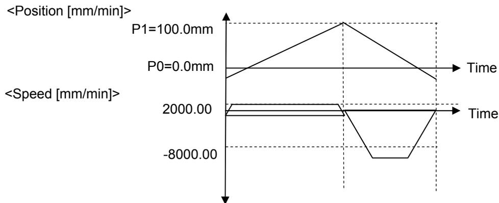
Positioning is started by setting the positioning start No. and turning ON the Positioning start signal.
