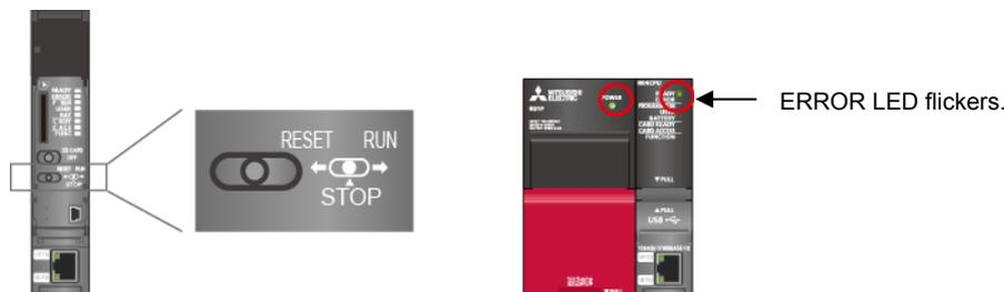
(a) Power supply module: LED (green light) turns ON.
