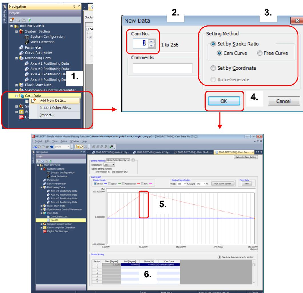
5. Make a rough cam graph by dragging an end of the cam waveform.
