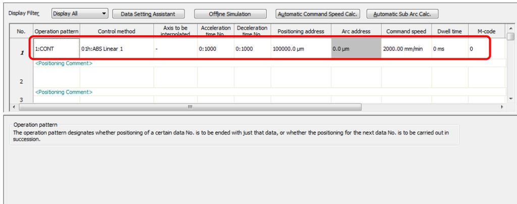
Create the positioning data in the same manner for the axis moving back to the home position from P1.
