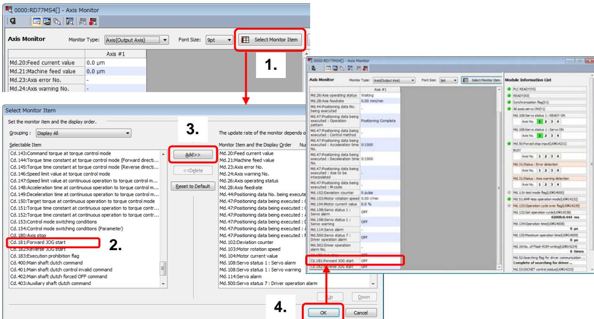
Check each status on the Axis Monitor window during JOG operation.
