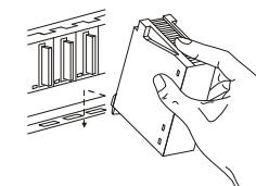
② Then press the module firmly into the base unit, making sure that it is fully inserted.
