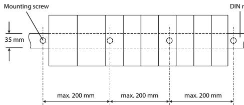
When installing the DIN rail in a large vibration and/or shock prone environment, insert the mounting screws in 200 mm intervals or less by the method shown below.
