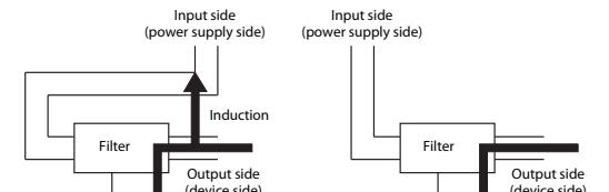
When the input and output wires are bundled, the noise will induct into the input side.
