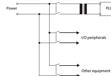
To minimize line voltage losses use cables with the maximum possible conductor cross-sectional area (max.  $2\ mm^2$ ) for the power supply lines. Install surge voltage protectors to protect the system against power surges (e.g. lightning strikes).
