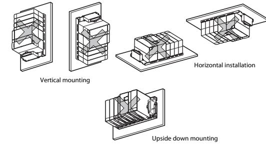
Avoid mounting of the base unit in proximity to vibration sources such as large magnetic contactors and no-fuse circuit breakers; mount these on a separate panel or at a distance. In order to avoid the effects of radiated noise and heat, provide the clearances indicated below between the PLC and devices that generate noise or heat (contactors and relays).
