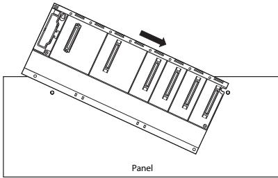
④ Slip the left mounting hole of the base unit over the other screw.
