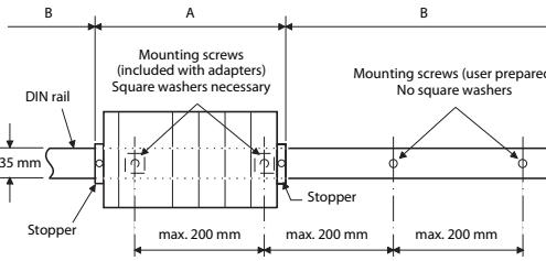
Insert the supplied mounting screws and square washers as shown below.
