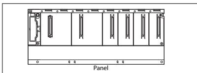
⑤ Insert the lower screws and tighten all screws to fasten the base unit to the wall.
