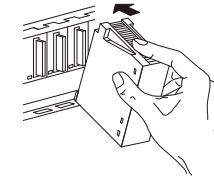
③ Secure the module with a fastening screw (M3 x 12) in installation locations where vibrations are expected. (Tightening torque: 0.36 to 0.48 Nm) These screws are not included with the modules.
