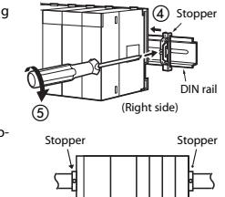
Make sure that the left and right stoppers are fixed securely to the DIN rail.
