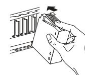
② Push the module in the direction of the arrow to load it into the base unit.
