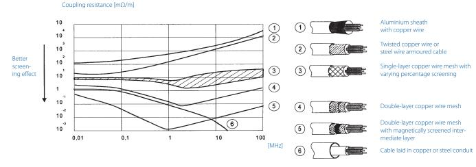
Coupling resistances for different types of screened cable
