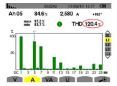
Input voltage and current of the inverter without the use of a harmonic-reducing input or DC link choke
