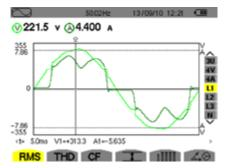
Input voltage and current when using an input choke and a DC link choke
