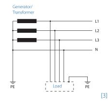
Industrial systems are usually supplied via transformers and dedicated distribution networks. Each network has its own EMC behaviour. The correct connection of an inverter therefore requires a knowledge of the existing network. The TN-S 5-conductor network provides the best situation, and the isolated IT network the worst.
