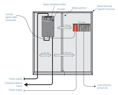
EMC-compliant installation of inverter
