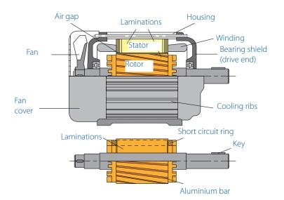
Longitudinal cut through a asynchronous motor
