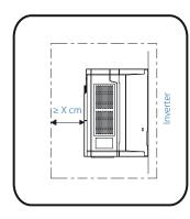
Minimum distances when installing the inverter in an electrical cabinet
