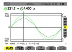
Input voltage and current when using a passive filter
