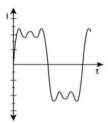
[2] Input current for a non-linear load
