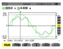
Input voltage and current when using a DC link choke
