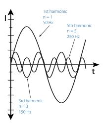
[3] Resulting sinusoidal oscillations (harmonics) of different frequency
