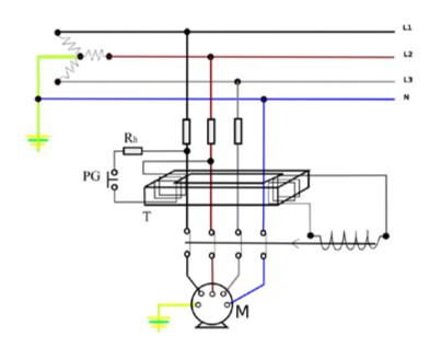
Principle of a 3-phase residual current device
