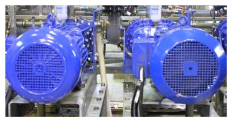
Self-ventilated motors for pump applications
