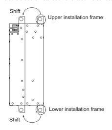
Installation of the multifunction regeneration converter in the enclosure Place the converter in an enclosure so that the converter's heat sink section protrudes from the hole through the panel of the enclosure. Fasten the converter to the panel with screws through holes in the upper and lower installation frames.
