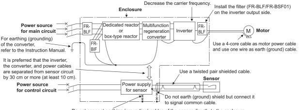
Do not connect earthing (grounding) cables of the sensor directly to the enclosure. Do not use control cables for earthing (grounding).
