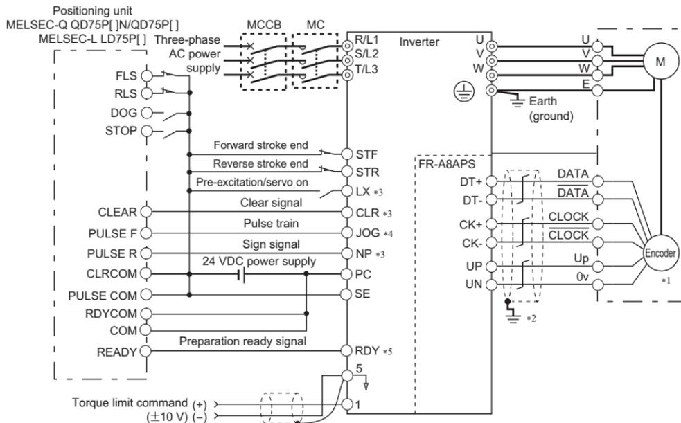
\*1 Connect the encoder so that there is no looseness between the motor and motor shaft. Speed ratio must be 1:1.
