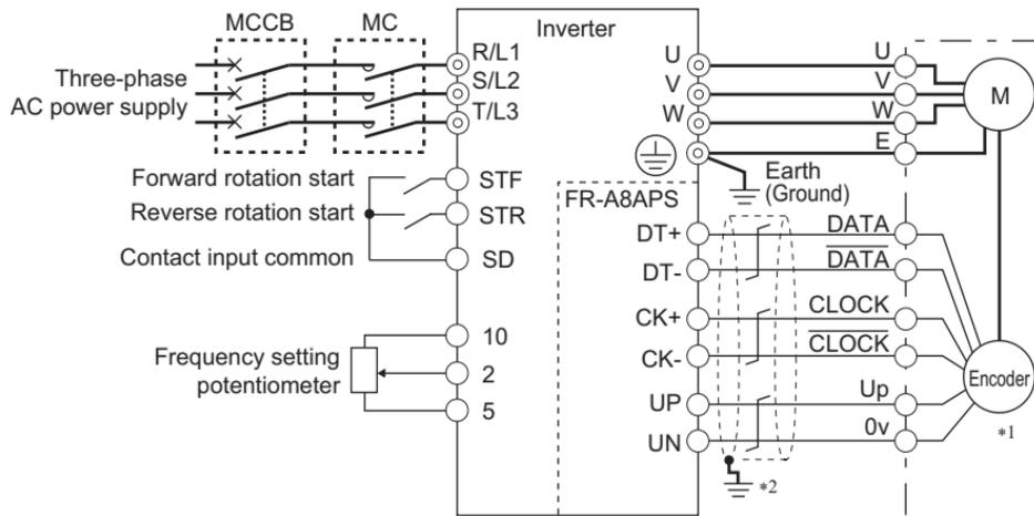
\*1 Connect the encoder so that there is no looseness between the motor and motor shaft. Speed ratio should be 1:1.
