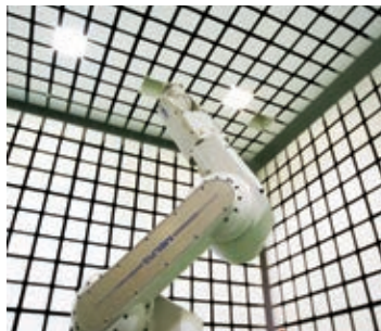
EMC chamber (large-size anechoic chamber)
