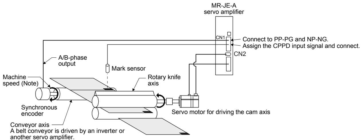
Note. Set the machine speed of the input axis to a value that satisfies the following equation.
