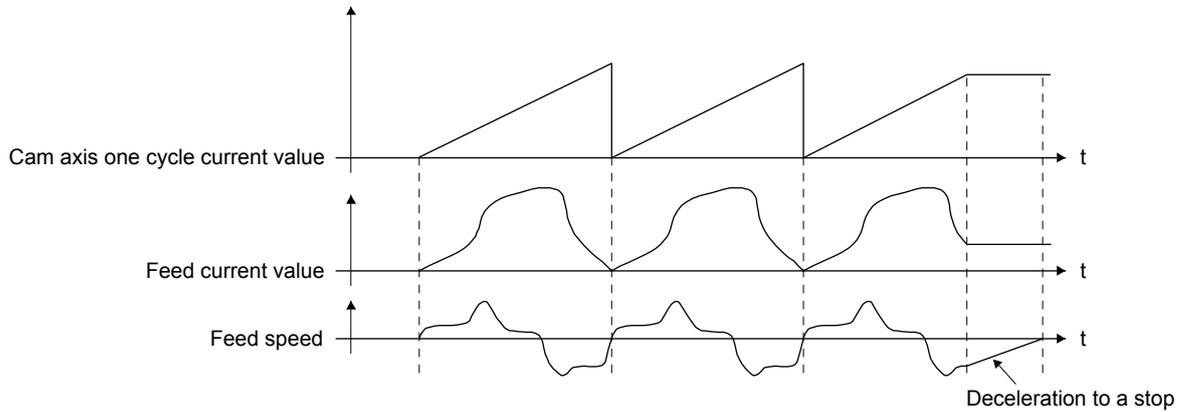
When using a positioning command (internal command) for the input axis, inputting a temporary stop or switching the operation mode decelerates the input axis to stop. Since the output axis stops in synchronization with the input axis, the synchronous relationship is kept and the cam control does not stop.
