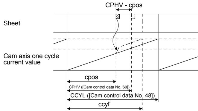
Increase the conveyor travel distance by adding the difference ( $CPHV - cpos$ ) to the cam axis one cycle current value. Adjust the filter time constant for acceleration/deceleration at compensation with [Cam control data No. 61 Cam position compensation time constant].
