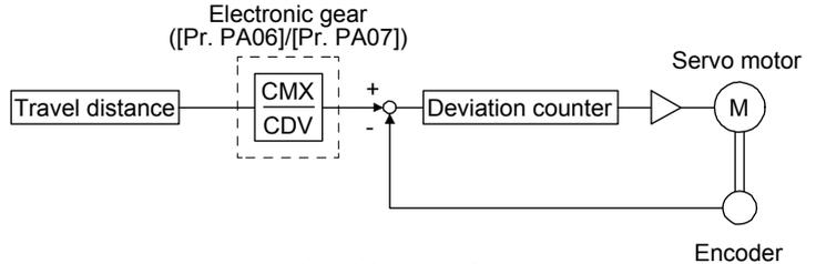
Pt: Servo motor encoder revolution 131072 [pulse/rev]
