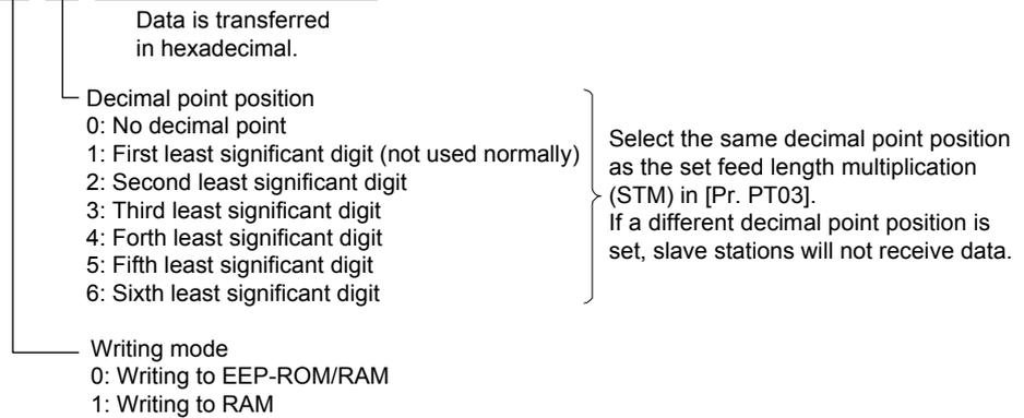
When changing the position data frequently using communication, set "1" to the write mode to change only the RAM data in the servo amplifier.
