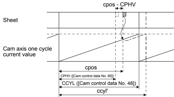
Decrease the conveyor travel distance by subtracting the difference ( $cpos - CPHV$ ) from the cam axis one cycle current value. Adjust the filter time constant for acceleration/deceleration at compensation with [Cam control data No. 61 Cam position compensation time constant].
