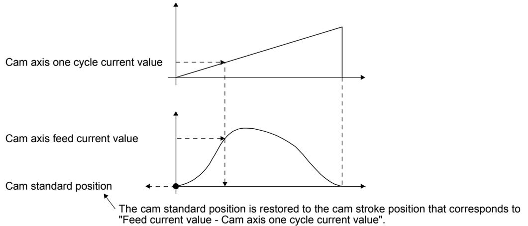
The following shows an example for restoring the cam standard position to start an operation from a point where both the feed current value and the cam axis one cycle current value are 0" in the cam whose cam data start position is not "0".
