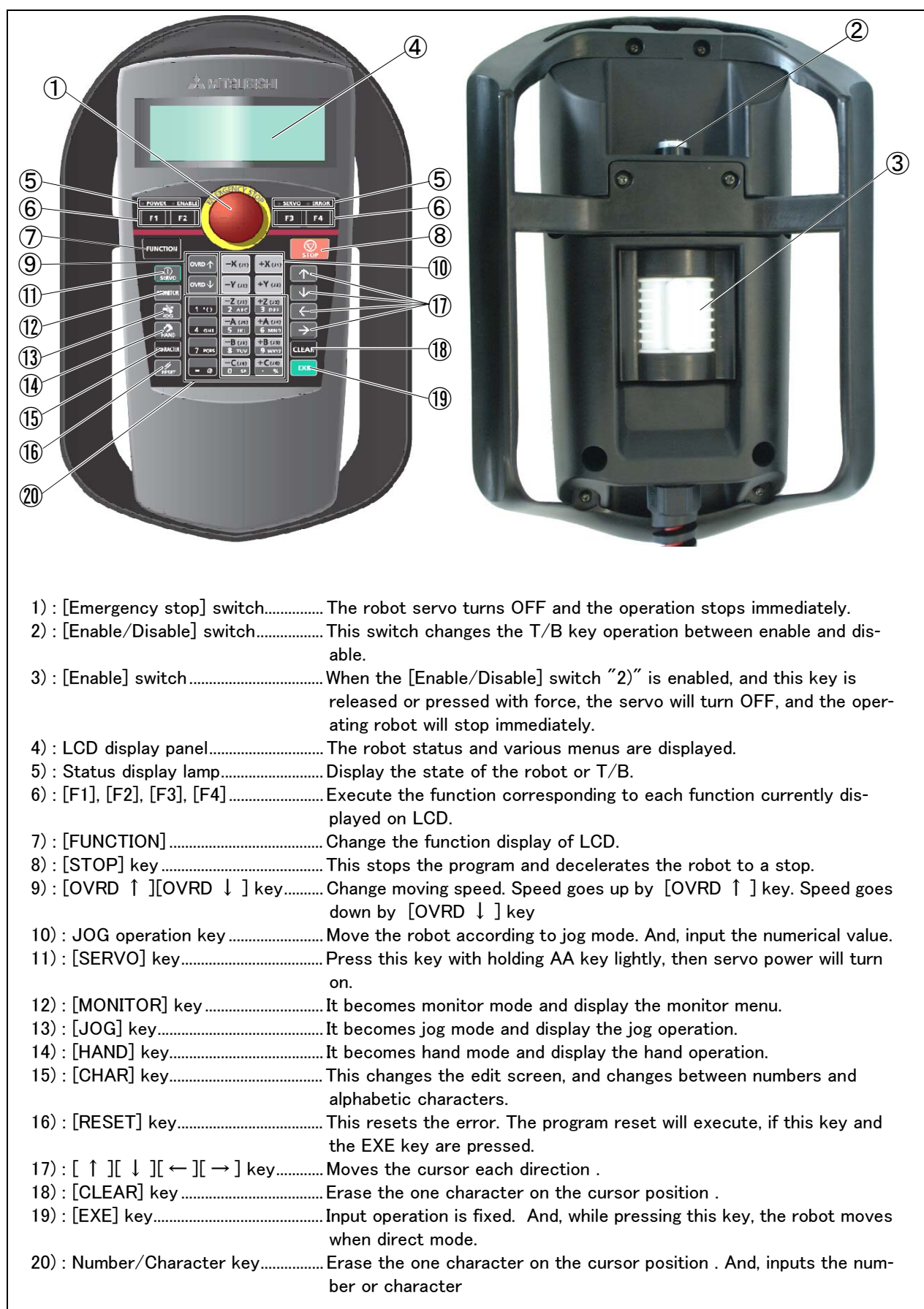
Fig.3-19 : Teaching pendant key layout and main functions
