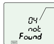
When incorrect wiring pattern cannot be detected
