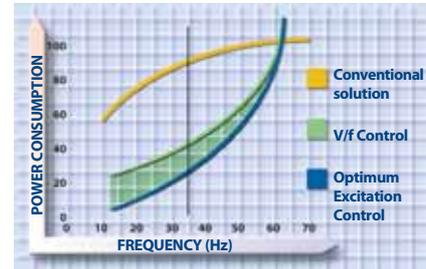
The inverter's energy saving capability is based on a principle called the cube law.
