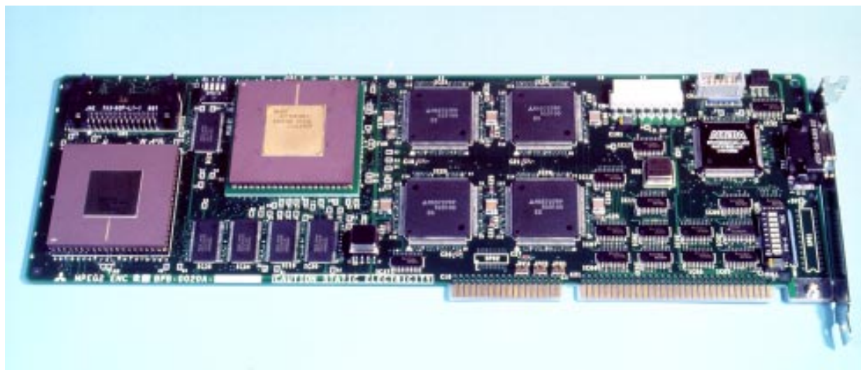
Fig.6 An MPEG2 encoder add-on board for personal computer use.
