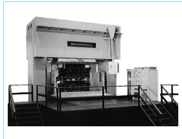
Fig. 2 A large, portal-type die sinker for draw dies.
