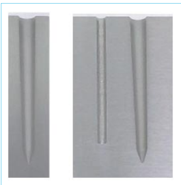
Fig. 7 High-speed test-cut sample for sub-gate pin holes
