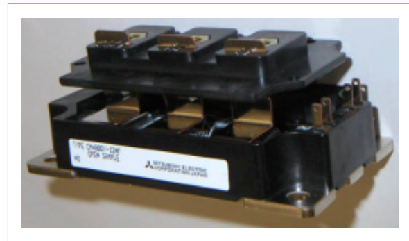
Fig. 2 An H Series-compatible cover on an F Series base case equals NF Series
