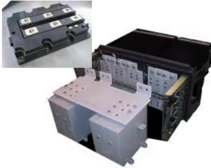
Fig. 1 IPM Device and Main Circuit Configuration
