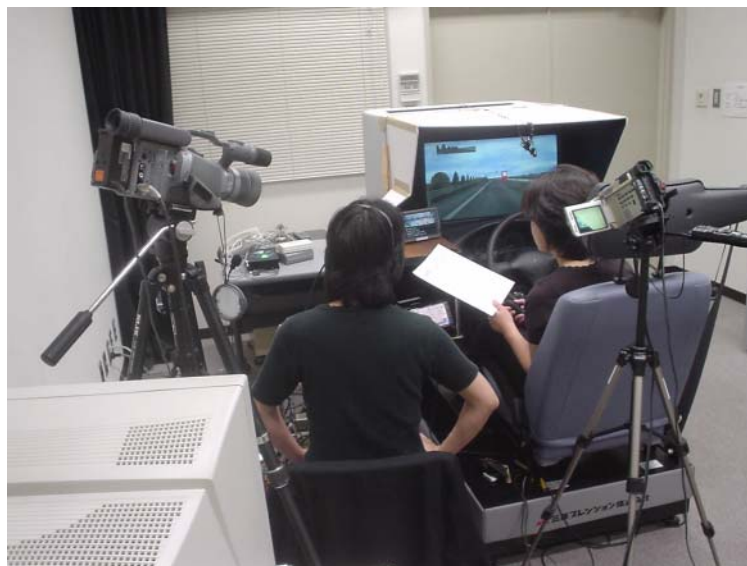
Fig. 1 User test using driving simulator
