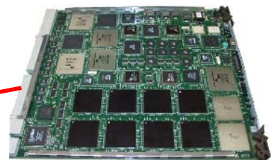
Baseband unit (Base station)
