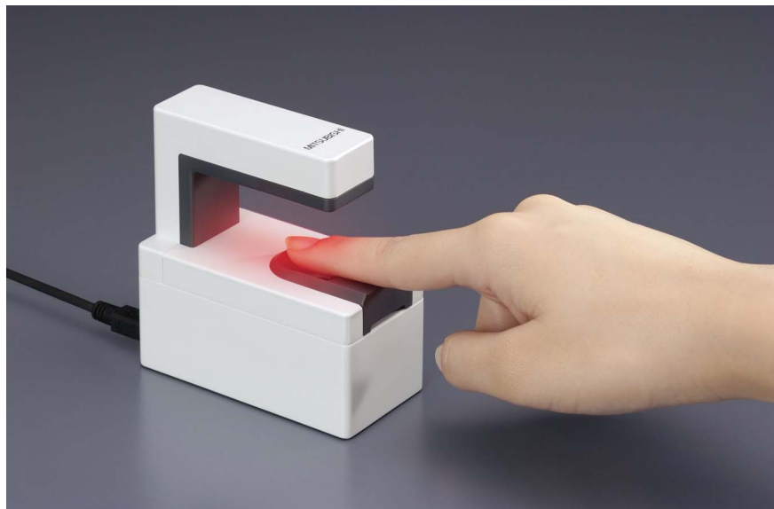
Fig. 1 Finger Identification Device By Penetrated Light (Desk Top Type)
