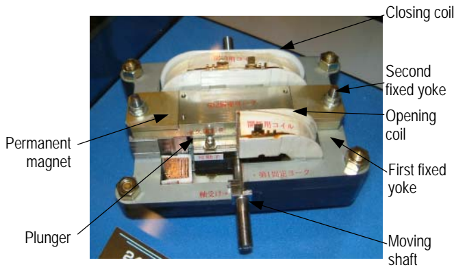
Fig. 2 Cut model of electromagnetic actuator
