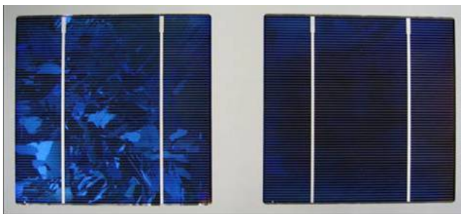
Fig. 2 Appearance of solar cells with an alkaline (left) and plasma (right) texture
