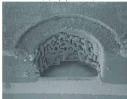
φ100-µm large window processing (Glass-epoxy resin)
