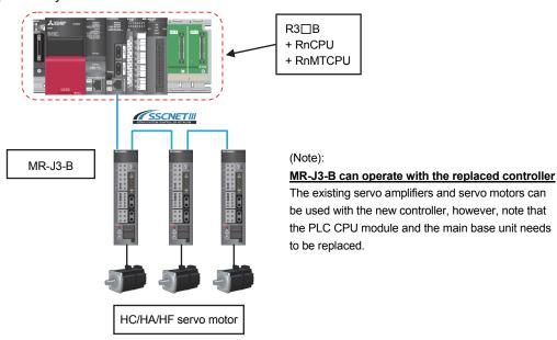
(2) When the MR-J3-B servo amplifier has malfunctioned. Replace only the servo amplifier.
