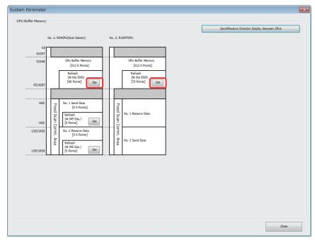
3) Set the following on the "Refresh (END) settings" screen below. When the refresh setting has been deleted, make the setting by referring to "Communication Area Setting (Refreshing Setting)" of MELSOFT GX Works2.
