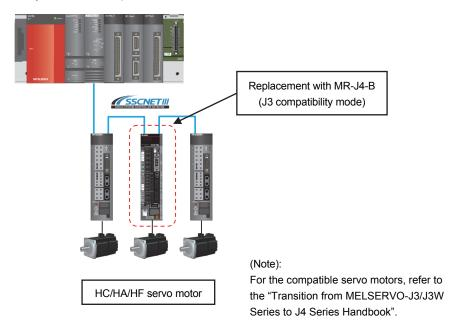
(3) When the HC/HA/HF servo motor has malfunctioned Simultaneously replace the servo amplifier and the malfunctioned servo motor.
