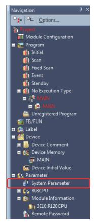
9) Select R120CPU in [I/O Assignment Setting] on "System Parameter" screen, and delete it with delete key. After the deletion, the multiple CPU setting is updated (R120CPU is deleted) by clicking one of the other tabs such as "Multiple CPU Setting" tab. Execute the procedure 9) through 11) successively.
